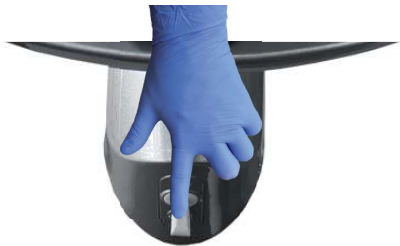
Composave setting on the joystick: Push forwards or backwards.
